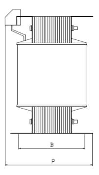
Technical data: Input 400.V at 50/60 Hz and Output 230.V Reference regulations: EN 61558-1 (CEI 96-1), EN 61558-2-13 (CE 14-8) Protection index: IP00 Ambient temperature: 35°C Thermal insulation class: B (130°C) The transformers are immersed in an insulating liquid Class "I": Grounding
